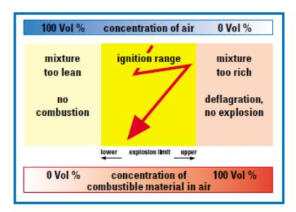
To avoid the danger of explosions, protective specifications in the form of laws, regulations, and standards have been developed in most countries, which are aimed at ensuring that a high level of safety is observed. In Europe (ATEX) and in the US legislation has been setup to minimise explosive atmospheres. As well as for manufacturers or equipment as for users of these equipment.
